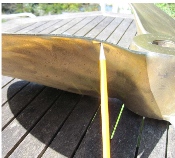
Two photos of Consuta's Propeller above – note the apparent change of pitch, all blades show this same bend in the blade form.
