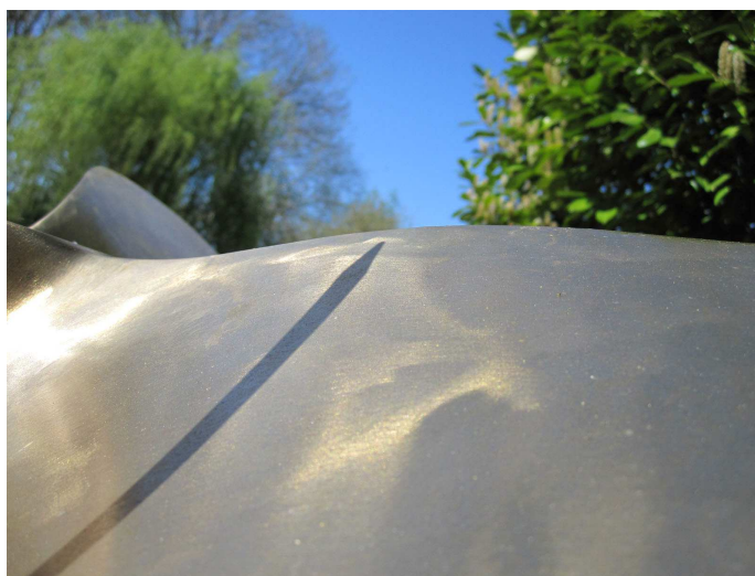
Two photos of Consuta's Propeller above – note the apparent change of pitch, all blades show this same bend in the blade form.
