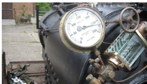
Water pressure at 270 psi
