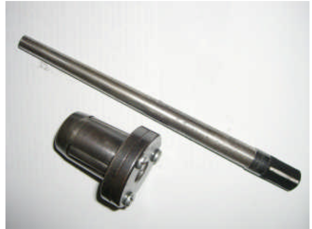
The tools used for fitting the replacement tubes. On the left is the reamer to make the tubes round and clean. On the right is the expander, the mandrel is rotated clockwise in its cage fitted in the tube end which slowly
