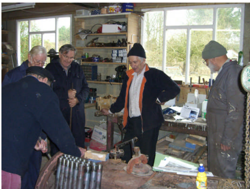
On the left the first part of the expanding operation can be done with an electric drill but the final expanding drive is manual using a torque lever because of the high torques needed and to get the right amount of tube expansion. The torque setting for these tubes was 50 ftlbs.
