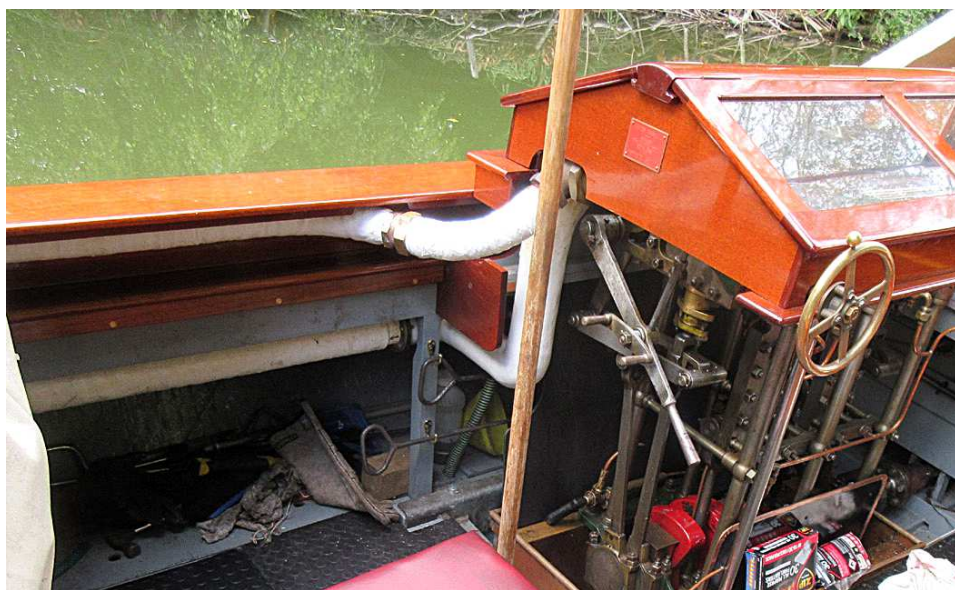
The engine pipe now lagged, lower pipe is engine 3" exhaust
