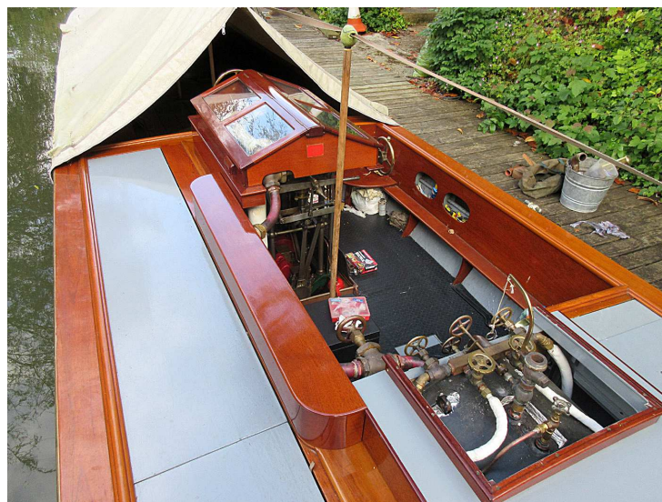
The wood cover over the engine steam pipe
