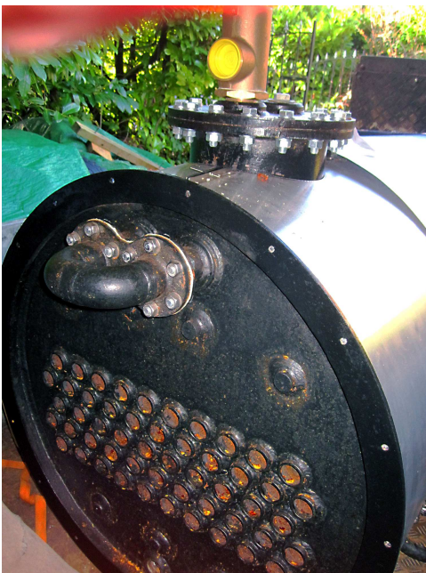
Front boiler tube plate Steam from the dome is looped back to the backhead, this is where a steam drier in the smoke box will be installed
