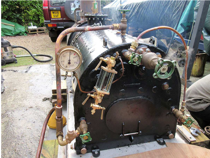
The new boiler without lagging under steam with minimal fittings being used - pressure is about 150 psi
