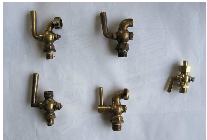
We've decided to try and find matching period drain taps for the engine. Not much available these days but the new one on the right is from China at a very reasonable price but not quite good enough. If you have anything like these in your junk box why not let us know - 1/4" BSP size.
