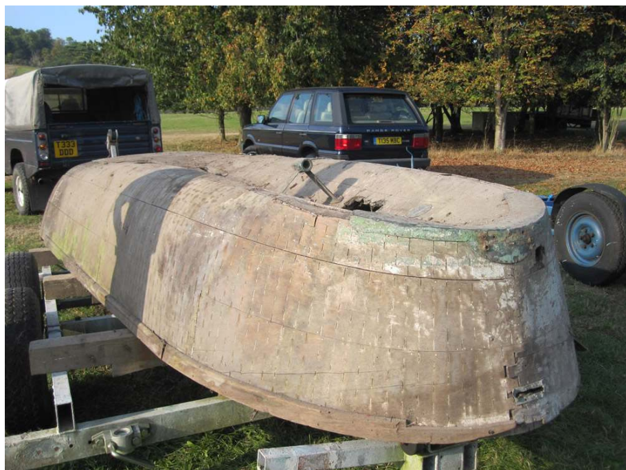
Photos of the stern part of Ulula, there is a centre section of about four feet missing.
