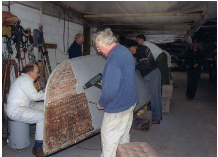
Geoff on paint removal work using a hot air gun and scraper
