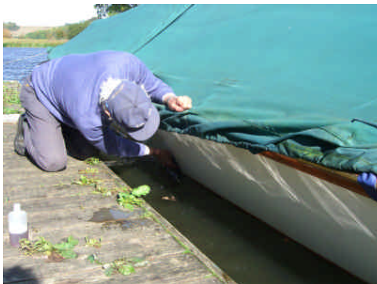
The Thames water seems to have been rather dirty this year. Using an acid cleaner to remove the grime along the waterline
